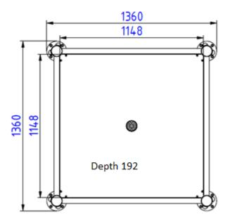
Fig. Dimensions of the elevated inclusive sandbox.
