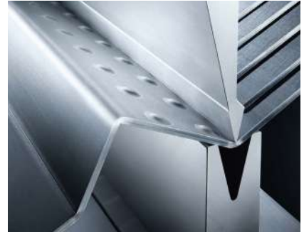
CNC steel plates bending
